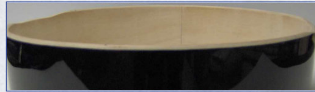
Custom bearing edge and snare bed cuts
